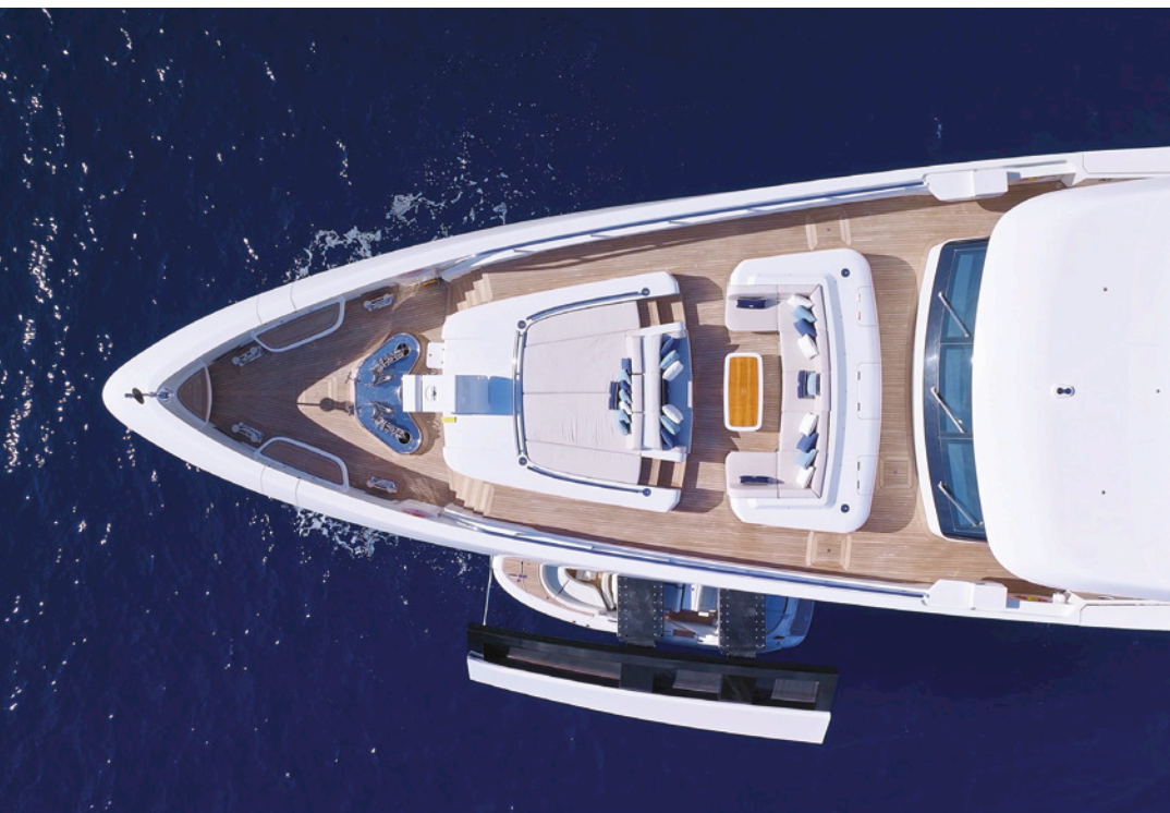
The main deck tender garage opens on both sides to free the Castoldi tenders or the WaveRunners. This design left room aft for a beach club
